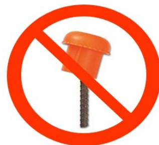
Figure 2: Typical example of an incorrectly fitted rebar-cap
